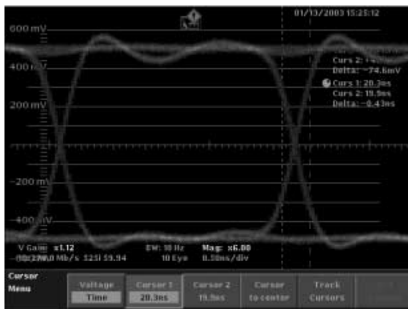
Figure 3-10: Timing Cursors alignment for measuring 20-80% rise time
